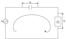
Applying KVL (Kirchof's voltage law), the calculated value of  $X_c$  is given by  $(V_s \times Z_F - V_F \times Z_F) / V_F = X_c$
