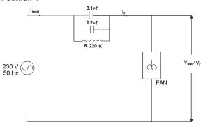
At this position, capacitor in the circuit  $3.1 + 2.2 = 5.3 \mu F$ .
