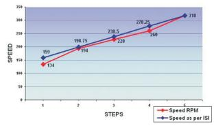
Type A fan tested on a standard regulator Case 3: Supply voltage = 240V
