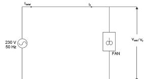
At this position there is no capacitor in the circuit and the fan moves at the full rated speed.
