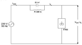
At this position, capacitor in the circuit =  $3.1 \mu$ F.
