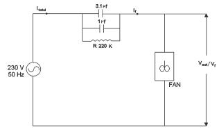
At this position, capacitor in the circuit =  $3.1 + 1 = 4.1 \mu F$ .
